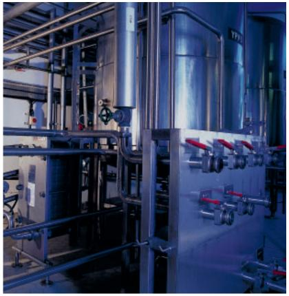
So we will carry them out regularly for you. A balanced test - at the maximum test pressure of the machine - will reveal any external leaks in the plate pack.
